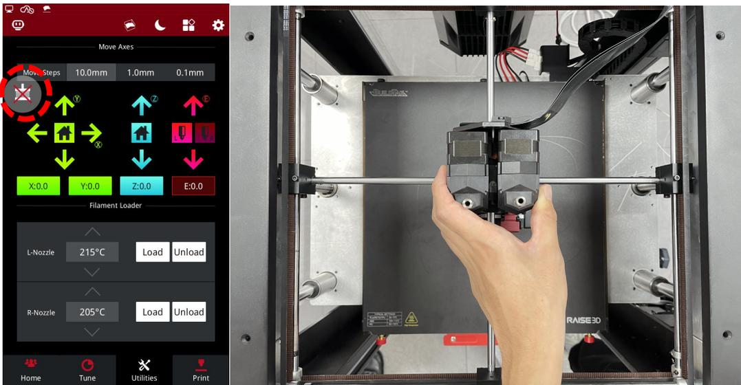
**Figure 1 Disable the motor and move the extruders to the center position.**
